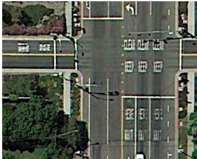
Additional Pavement Markings
