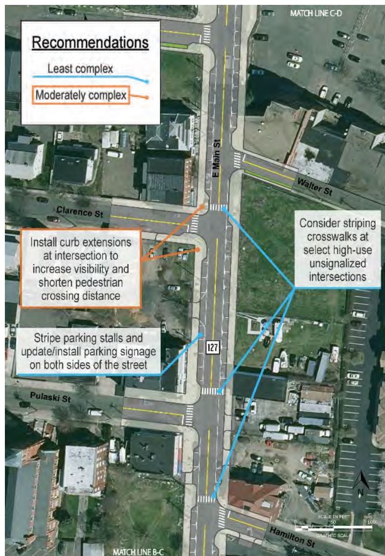
Exhibit 24: Location C (Hamilton Street to Crescent Place)
