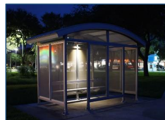
Figure 10: An internally illuminated bus shelter powered by solar.
