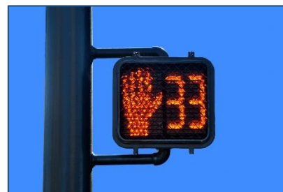
Figure 8: A crosswalk countdown signal showing the time left in a pedestrian crossing phase.
