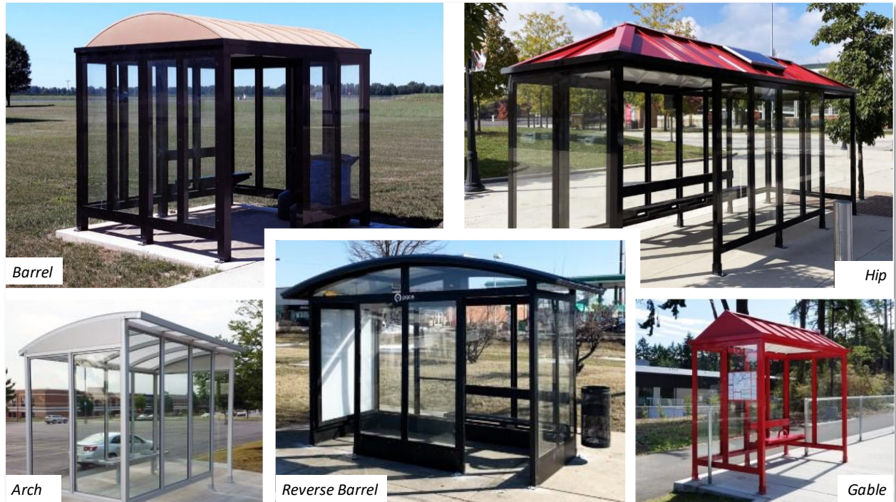
Figure 12: The palette of bus shelter roof styles selectable through the Bus Stop Enhancement Program
